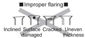
When properly flared, the internal surface of the flare will evenly shine and be of even thickness. Since the flare part comes into contact with the connections, carefully check the flare finish.
