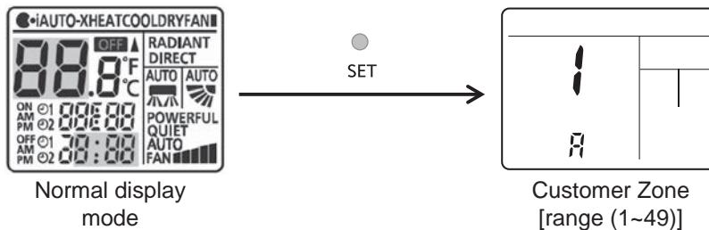
4 To enter Service zone: (Press **SET** continuously for  $T \geq 5$  secs)
