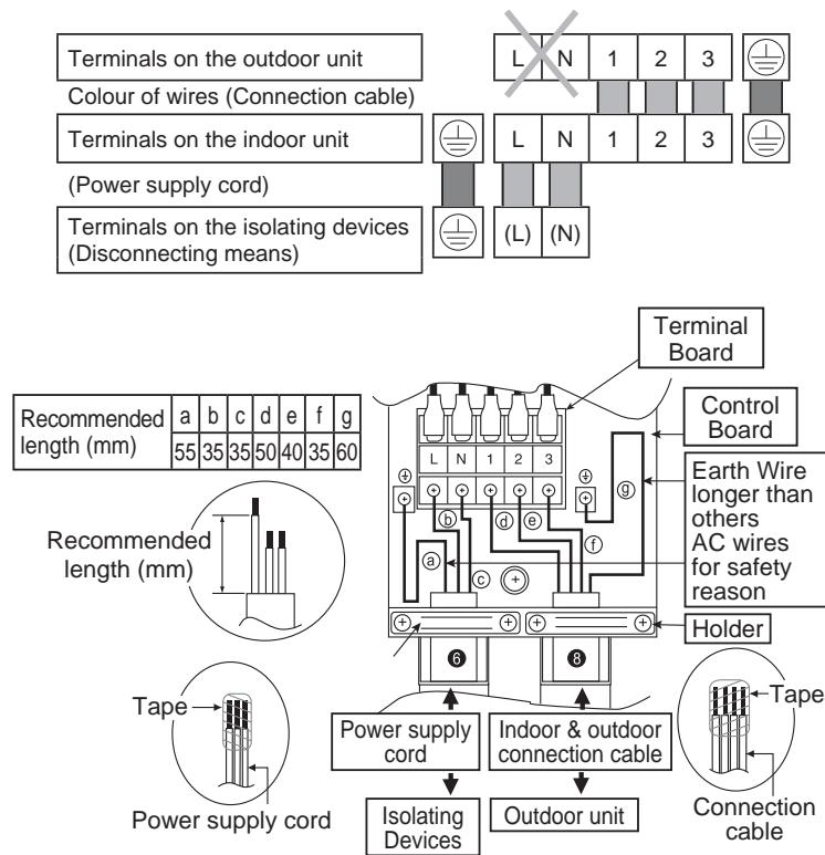
10 Secure the power supply cord and connection cable onto the control board with the holder.
