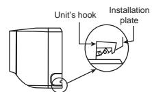
To take out the unit, push the **PUSH** marking at the bottom unit, and pull it slightly towards you to disengage the hooks from the unit.
