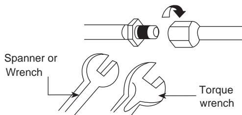
Additional Precautions For R32 Models when connecting by flaring at indoor side
