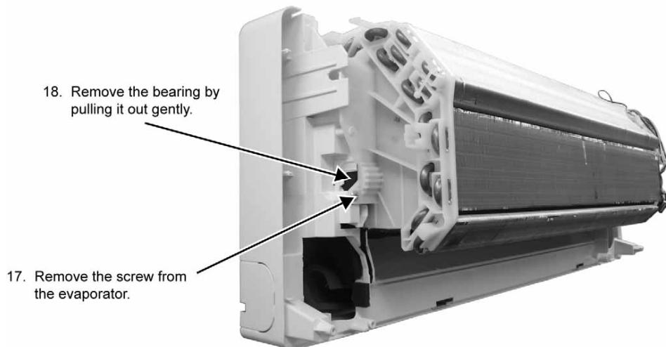
17. Remove the screw from the evaporator.
