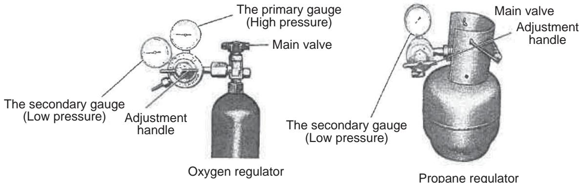
2. Open the cylinder valve, and check the remaining amount with the first t side pressure gauge.
