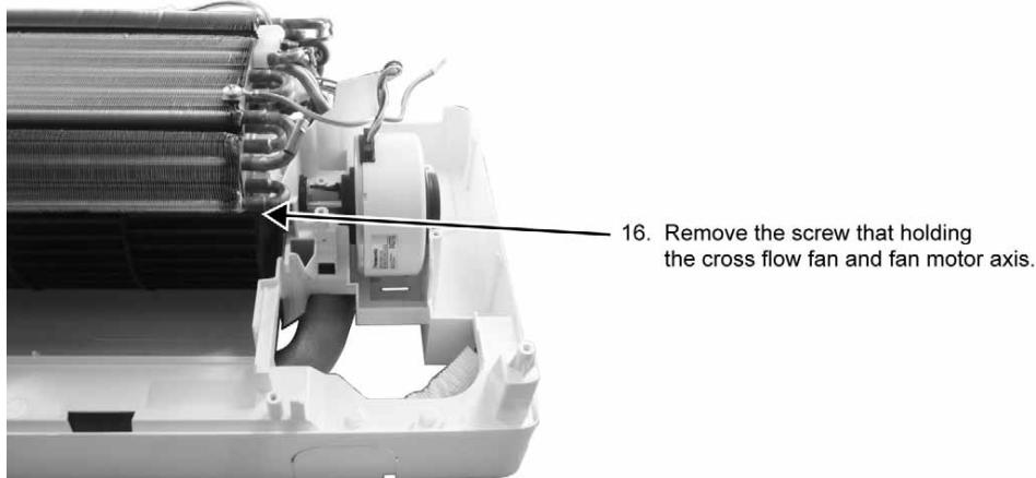
16. Remove the screw that holding the cross flow fan and fan motor axis.
