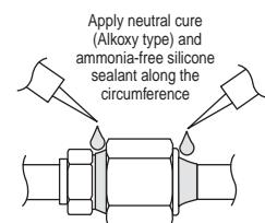
Neutral cure (Alkoxy type) & ammonia-free silicone sealant is only to be applied after pressure testing and cleaning up by following instructions of sealant, only to the outside of the connection. The aim is to prevent moisture from entering the connection joint and possible occurrence of freezing. Curing sealant will take some time. Make sure sealant will not peel off when wrapping the insulation.
