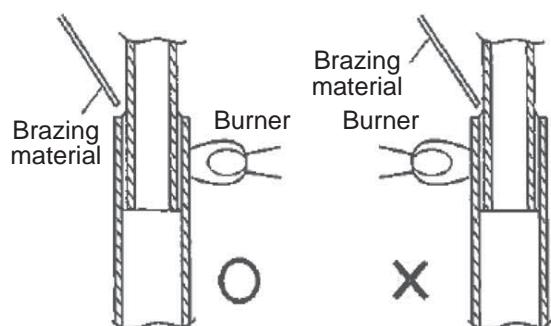
The pre-heating is to heat the base material until the melting temperature, and requires certain training to distinguish the color of the heated base material in order not to melt the material.
