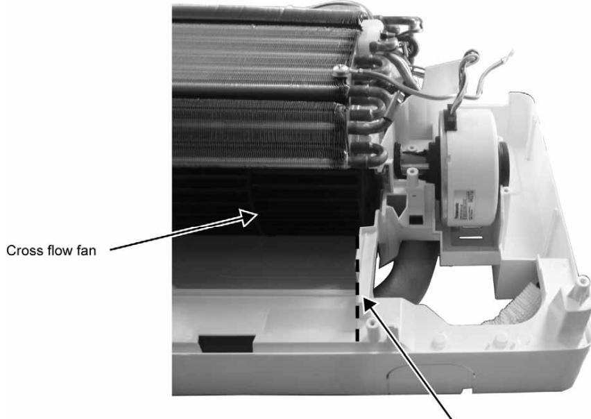
Reminder: To reinstall the cross flow fan, ensure cross flow fan is in line as shown in figure 12.
