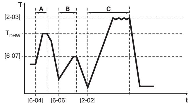
**A** Scheduled storage operation: activated at [6-04], heat up domestic hot water until domestic hot water user interface set point  $T_{\text{DHW}}$  (e.g.  $55^{\circ}\text{C}$ ) is reached.
