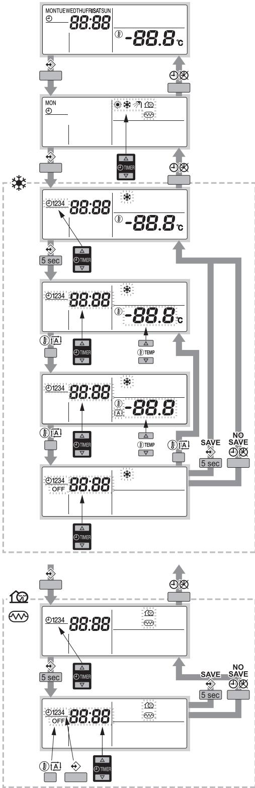
Programming space cooling, quiet mode, or booster heater mode<sup>(1)</sup> is carried out as follows:
