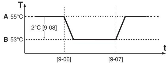
A Normal leaving water temperature set point or calculated weather depended set point
