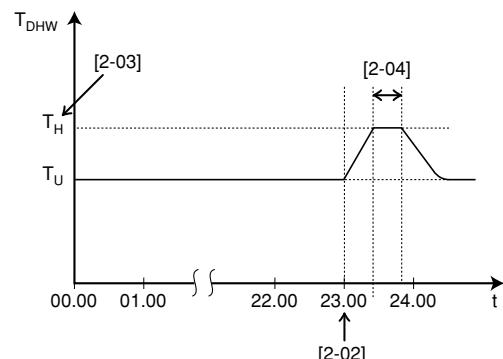
$T_{DHW}$  Domestic hot water temperature
