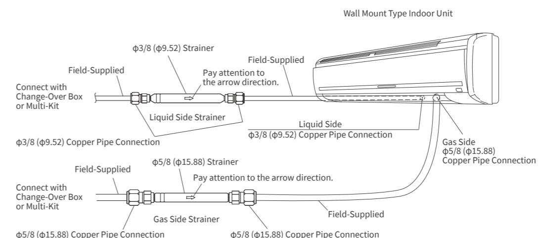
Insulate all the refrigerant piping to prevent condensation. If piping is exposed to the ambient atmosphere, dew condenses over the piping surface and water drips. In an instance where the piping size does not correspond with the strainer kit, use a reducer(field-supplied).
