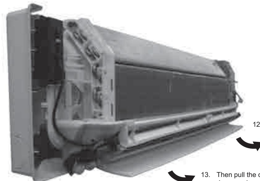
12. Pull out and remove the drain hose from the discharge grille.
